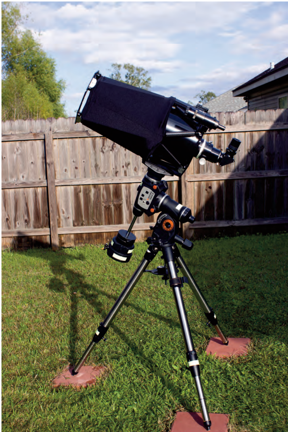
Image 11 - The 40-pound capacity Celestron CGEM II mount handles the OTA adequately for visual use and lunar and planetary imaging. A larger capacity mount would be needed for long-exposure digital imaging.
