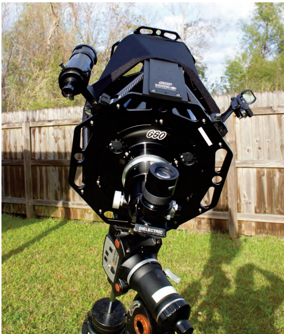
Image 10 - The telescope comes with two finder shoes where I have attached a red dot finder and a 9x50 finderscope. The second Losmandy-style dovetail plate on top of the OTA can be used for attaching a guide scope.
