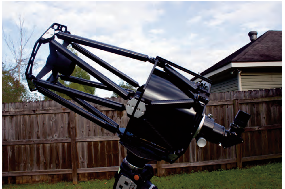
Image 1 - Unlike the 6-inch and 8-inch version, the GSO 10-inch classical Cassegrain telescope has a truss tube design making it lighter and giving it better thermal characteristics. The trusses are made of low thermal expansion carbon fiber tubes.
