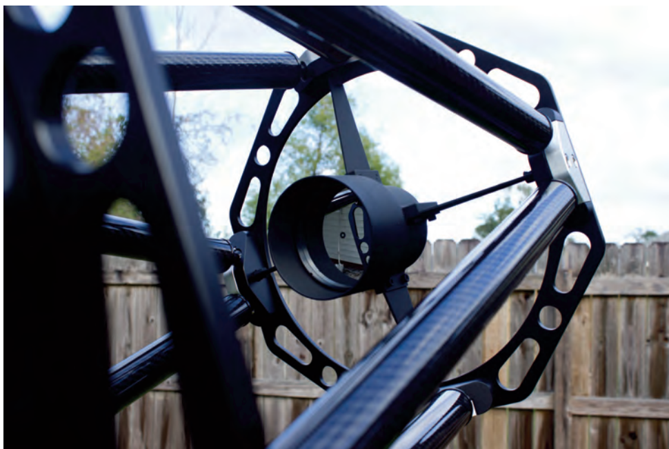
Image 4 - This view shows the secondary mirror. It is well shielded and also center marked for collimation.
