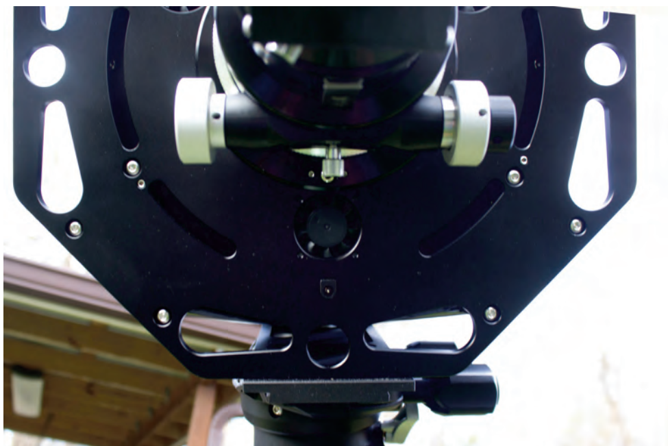
Image 6 - The 12V jack for powering the mirror cooling fans is found below the focuser and lower cooling fan.
