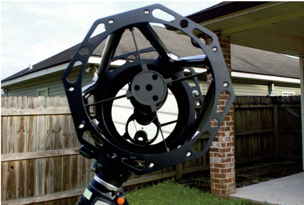
Image 3 - The primary mirror is center marked for use in collimation.
