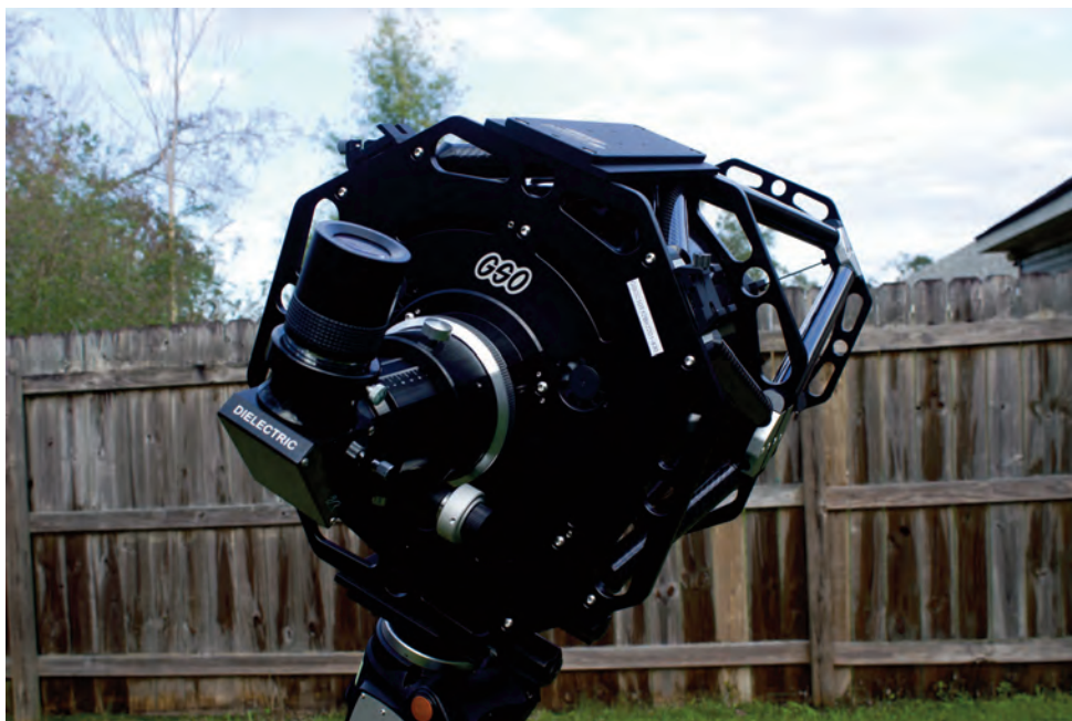
Image 5 - The backside of the telescope showing the focuser, cooling fans and primary mirror collimation screws.
