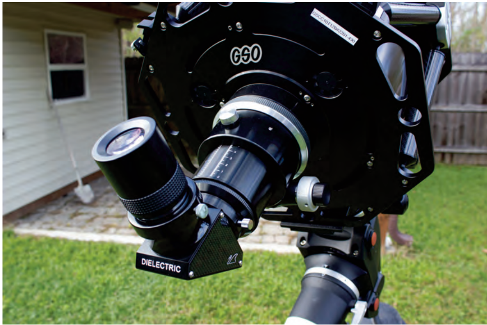
Image 7 - The telescope comes with a 3.25-inch dual speed focuser with a graduated 2-inch drawtube.
