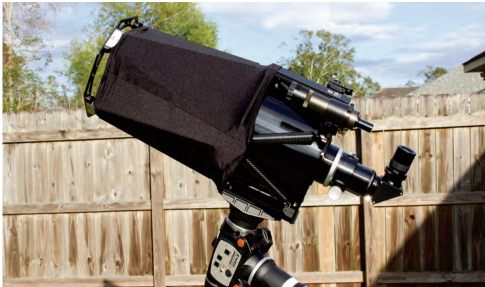
Image 9 - I had a custom shroud made to keep dew, stray light and dust out of the OTA when in use.
